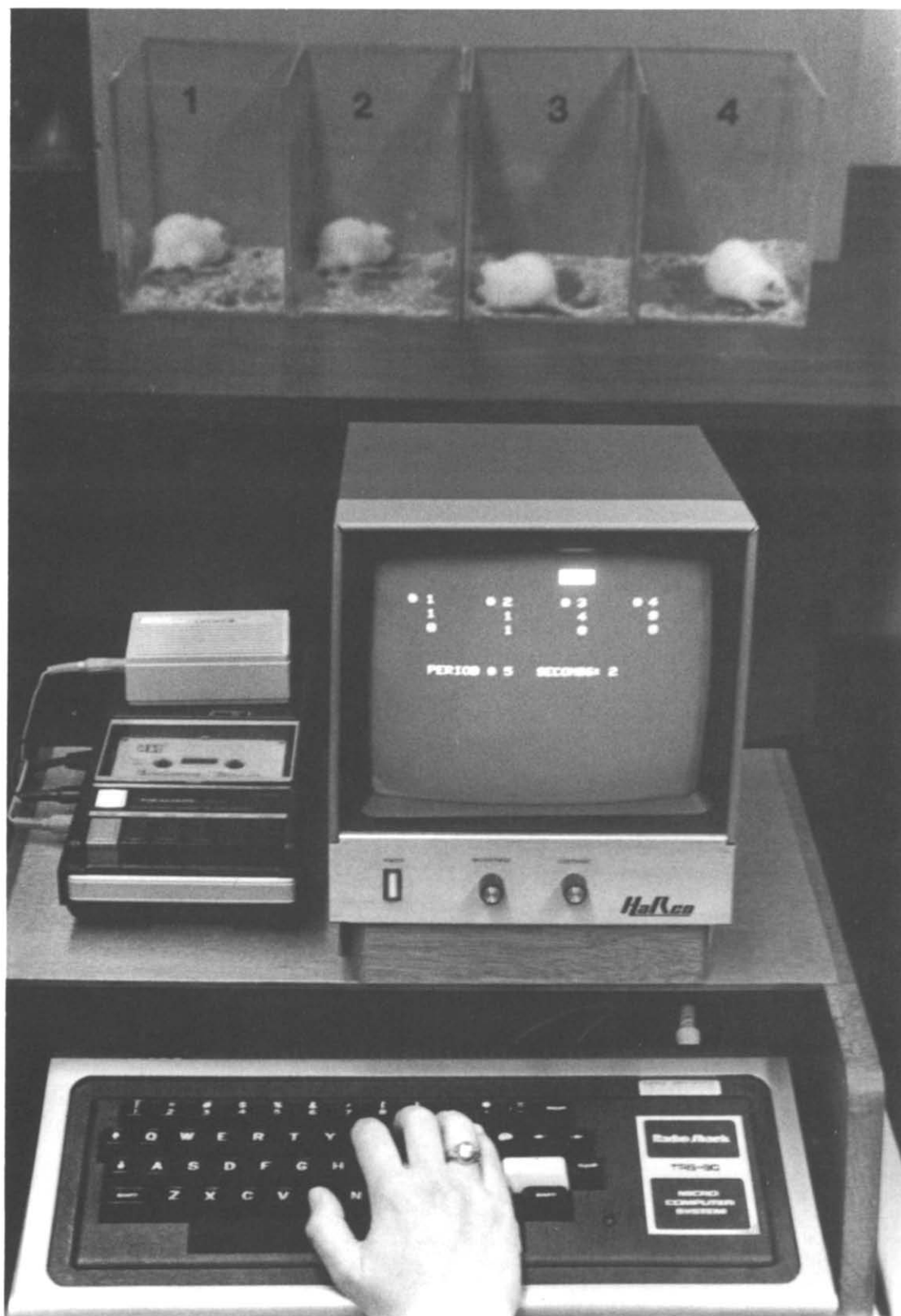
FIG. 1. The experimental set-up; note video graphic "flag" used to prompt the user to observe animal 3. The screen shows cumulative total of behavior 1 (middle row of numbers) and occurrence of behavior 2 in the current observation period (bottom row).
